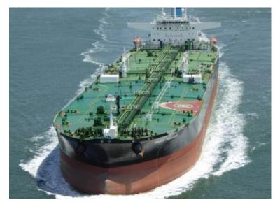
The term 'Suezmax' refers to the largest ships capable of travelling along the Suez Canal, and generally refers to tankers.
